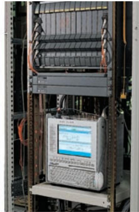
ANT-20E used as ATM tester at German network provider “tesion”. More about broadband applications in our next issue of Advanced Network Testing.
